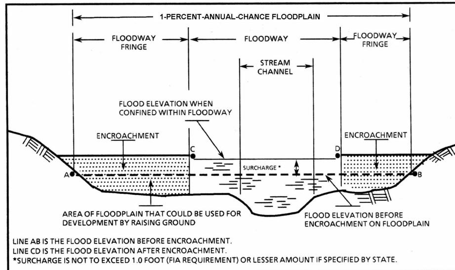
Figure 1. Floodway Schematic
