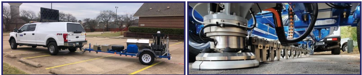
Figure 12 - Fast Falling Weight Deflectometer
