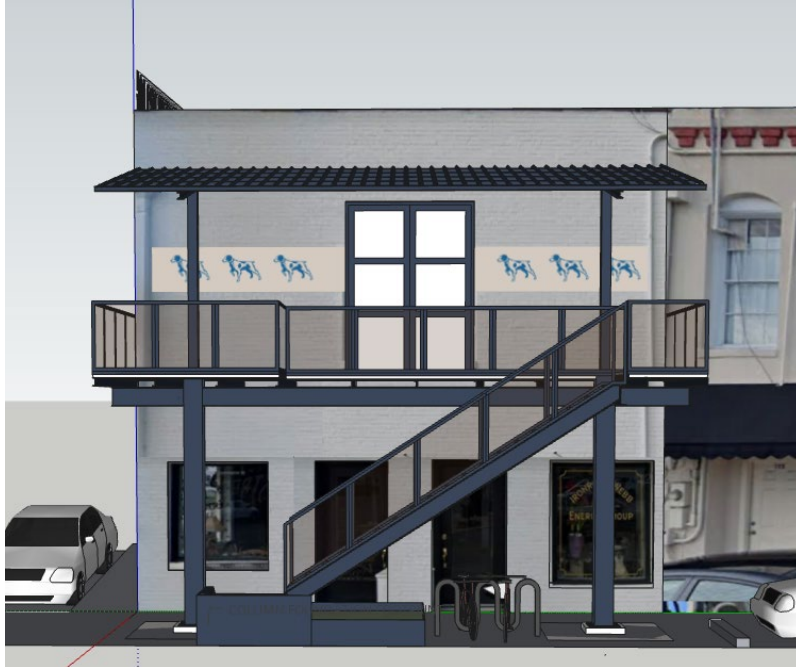
Figure 3 Proposed Balcony and Stair Structure
